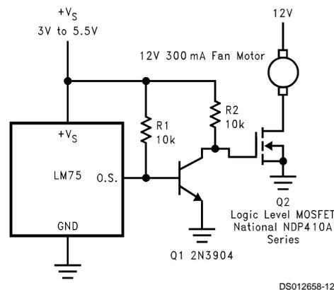
When using the two-wire interface: program O.S. for active high and connect O.S. directly to Q2's gate.
