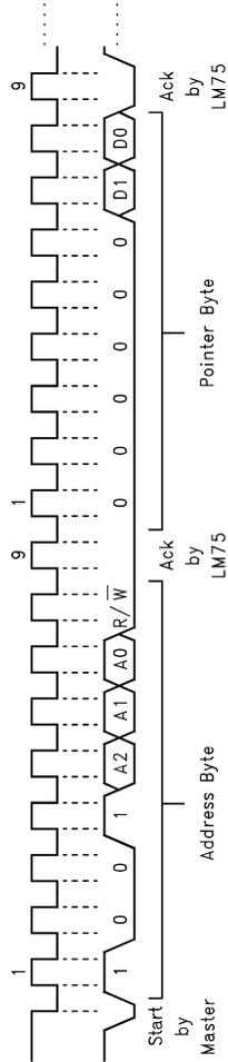
(b) Typical Pointer Set Followed by Immediate Read for 2-Byte Register such as Temp,  $T_{OS}$ ,  $T_{HYST}$
