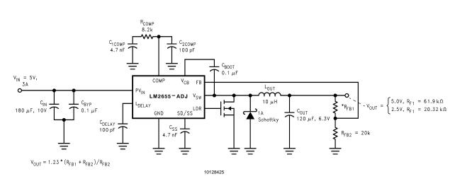
FIGURE 3. Programmable output voltage.
