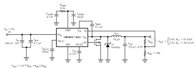
Schematic for the Typical Board Layout
